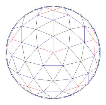
Those three strut sizes are used to make two types of triangles, ABA and CBC triangles. Both are isosceles triangles, meaning that two sides are equal in length and two angles are equal. These two triangle types are assembled into pentagons and hexagons, each with a raised center. The ABA triangles form pentagons (red surrounded by blue) and the CBC triangles form hexagons (black surrounded by blue). For a 5/9 truncation dome there are six pentagons and ten hexagons, and five half hexagons.
