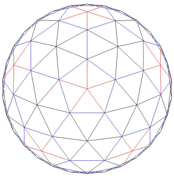
While a 3v dome appears to be complicated when you look at all the individual elements, it is actually very simple. In the above picture you can see red struts, blue struts, and black struts. There are only three lengths of struts in a 3v dome. We call the red, or shortest struts, "A". The blue, middle sized struts are "B", and the black longest struts are C".
