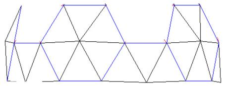
The hubs at the bottom and the centers of the hexagons are complete and can now be tightened to their final torque.
