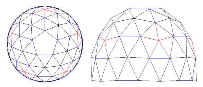
8. Install the last pentagon module at the top of the frame and tighten its center and surrounding B struts.
